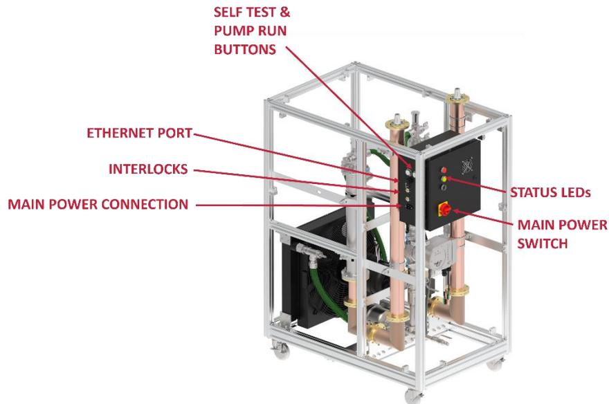
Figure 5: Components of the electrical box
