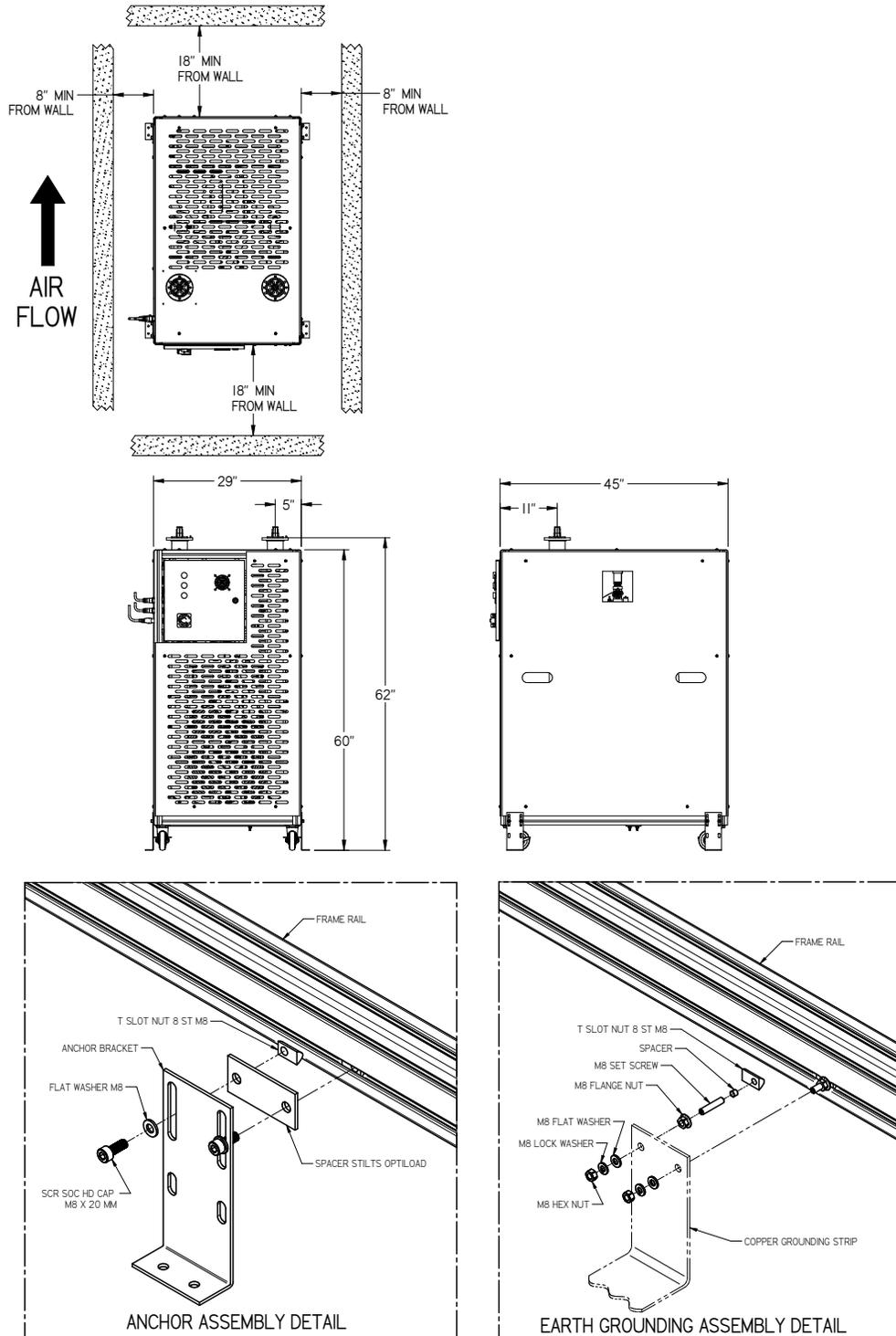
Figure 10: Positioning, anchoring, and grounding steps
