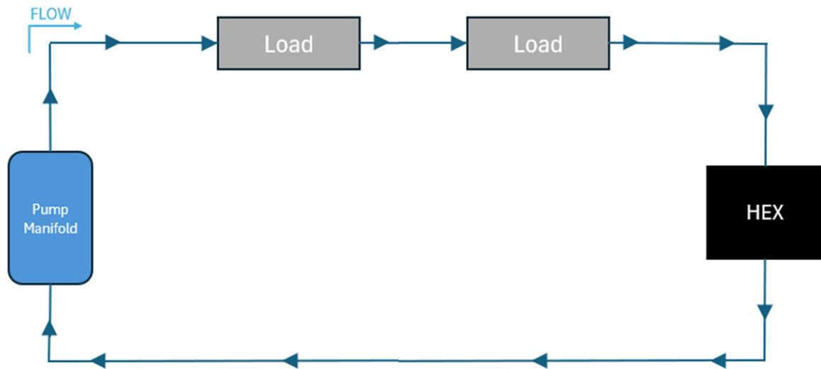
Figure 9: Direction of coolant flow through the system
