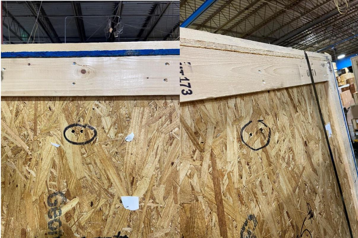
Figure 23: Screws to be removed on the front and rear panels of crate to remove internal cross support
