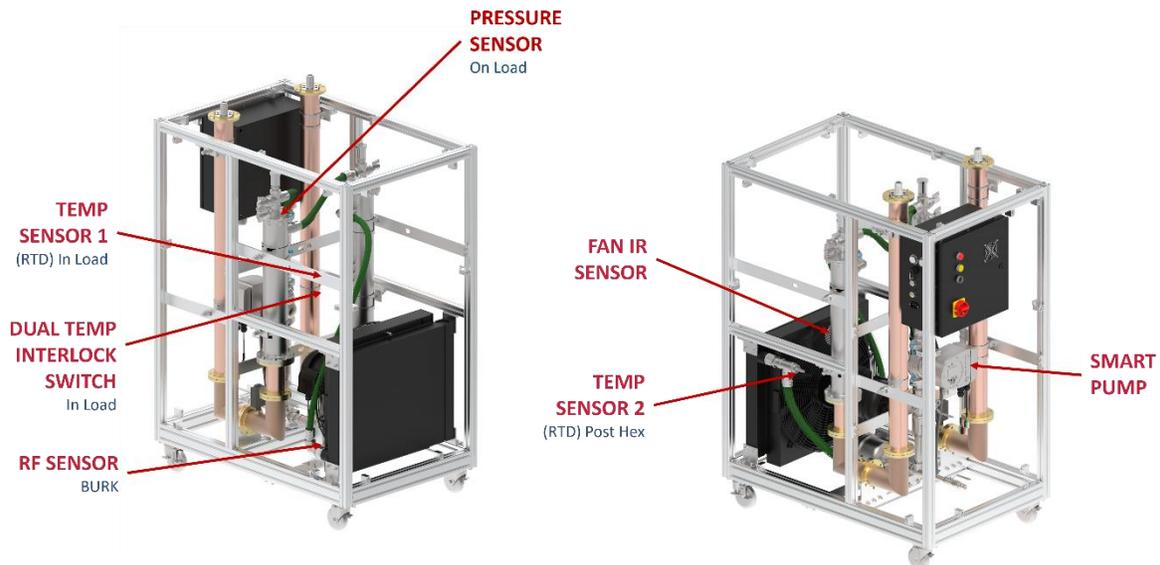
Figure 4: Placement of sensors
